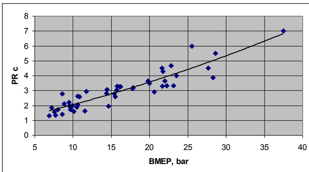
Figure. 1. Dependence of the compressor pressure ratio PRc at nominal RPM on BMEP.
