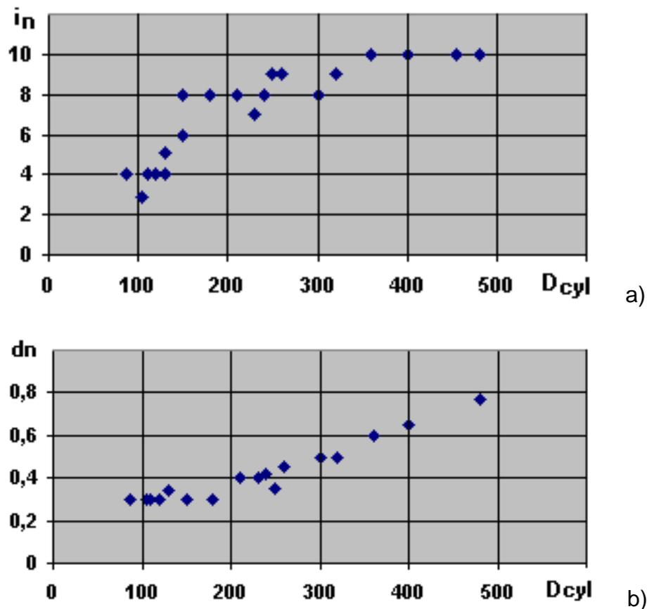
Fig. 4. Dependence of (a) nozzle number,  $i_n$ , and (b) orifice diameter,  $d_n$  [mm], on cylinder diameter  $D_{cyl}$  [mm].
