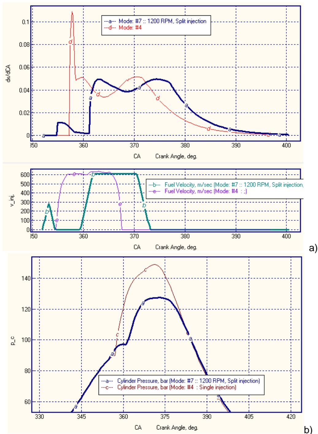
Figure 22. Comparison of (a) the rate of heat release and (b) in-cylinder pressure with single and double injections at 1200 RPM.
