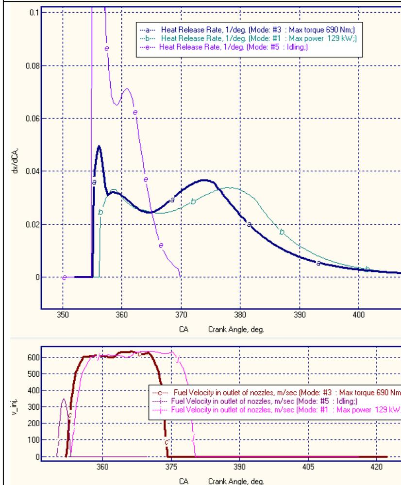
Figure 14. Comparison of the rate of heat release,  $dx/CA$ , and the fuel injection velocity,  $V_{inj}$  [m/s], as a function of RPM. The highlighted line corresponds to the maximum torque regime.
