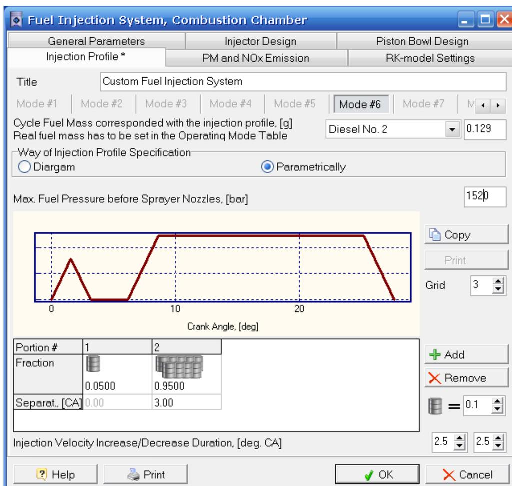
Figure 18. Settings for the injection characteristics with common rail system for regime No. 6 (maximum torque at 1500 RPM).
