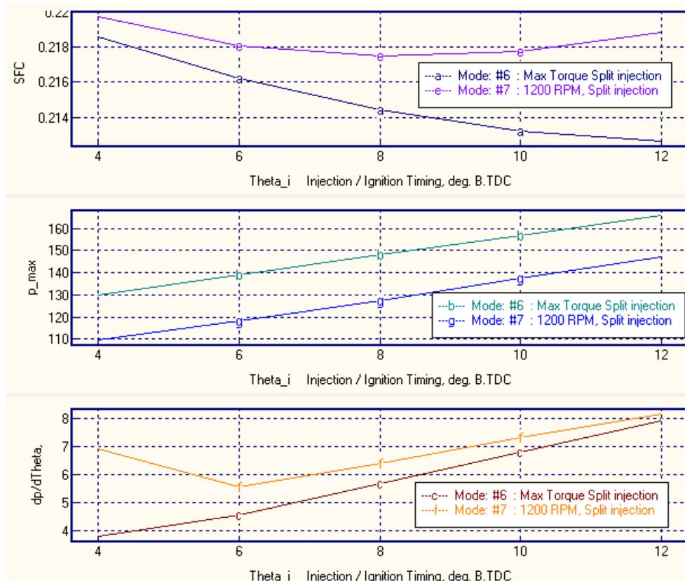
Figure 20. The effect of the injection timing  $\Theta_{i}$  on engine parameters at regime No. 6 (1500 RPM) and No. 7 (1200 RPM).
