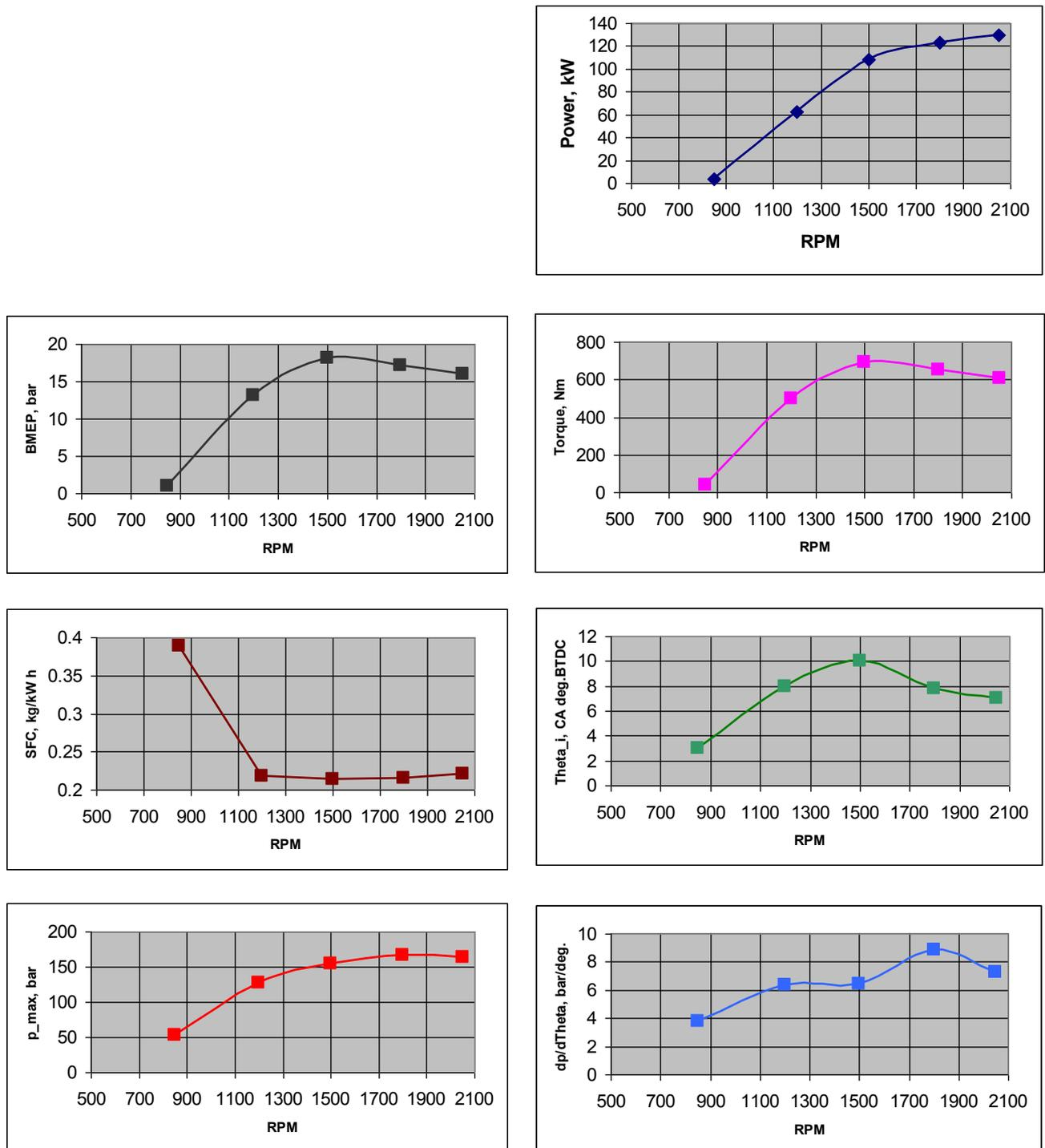
Figure 21. Engine operating parameters with fuel multiple injection for diesel output characteristics.
