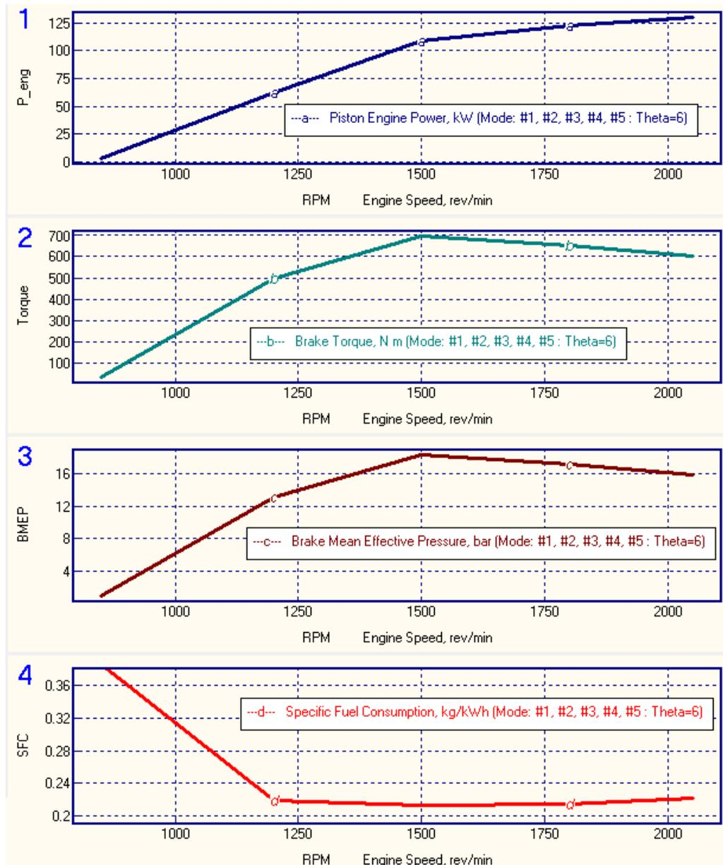
Figure 11. The change of engine parameters vs. RPM: (1) Power,  $P_{eng}$  [kW], (2) Torque,  $Torque$  [Nm], (3) Brake mean effective pressure,  $BMEP$  [bar], (4) Specific fuel consumption,  $SFC$  [g/kWh]
