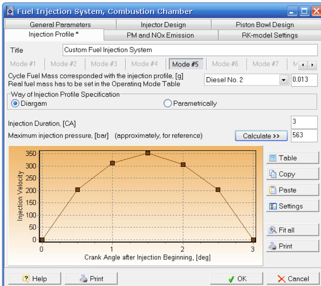
Figure 7. Fuel injection characteristics at engine idling regime.
