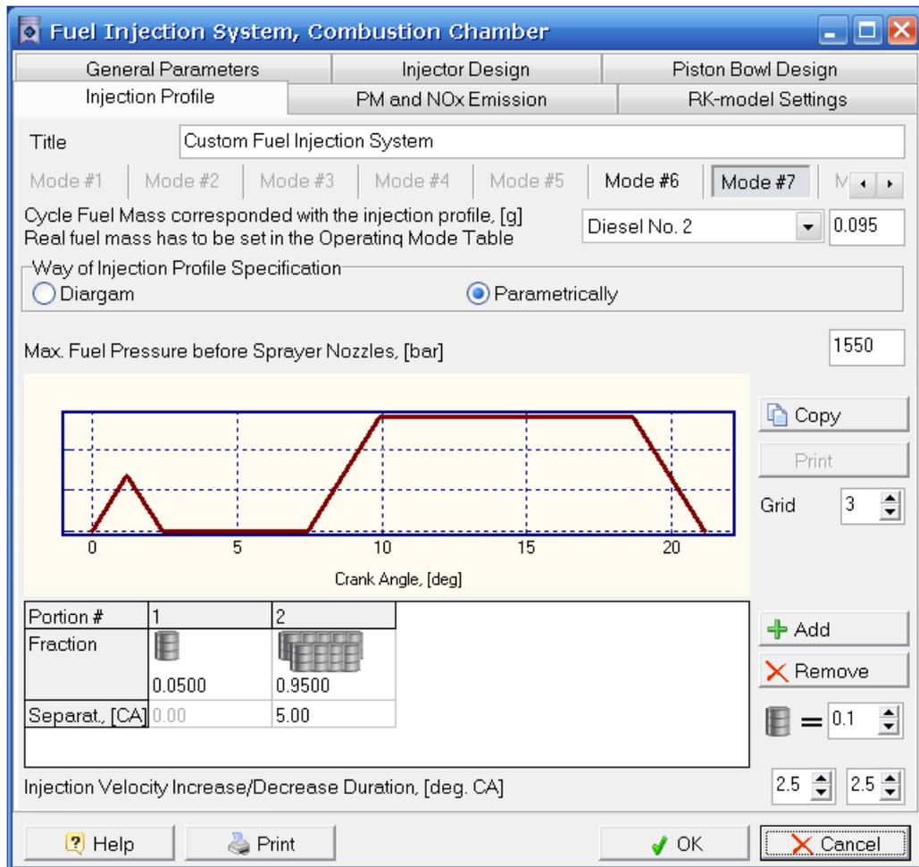
Figure 19. Settings for the injection characteristics with common rail system for regime No. 7 (lower engine speed at 1200 RPM).
