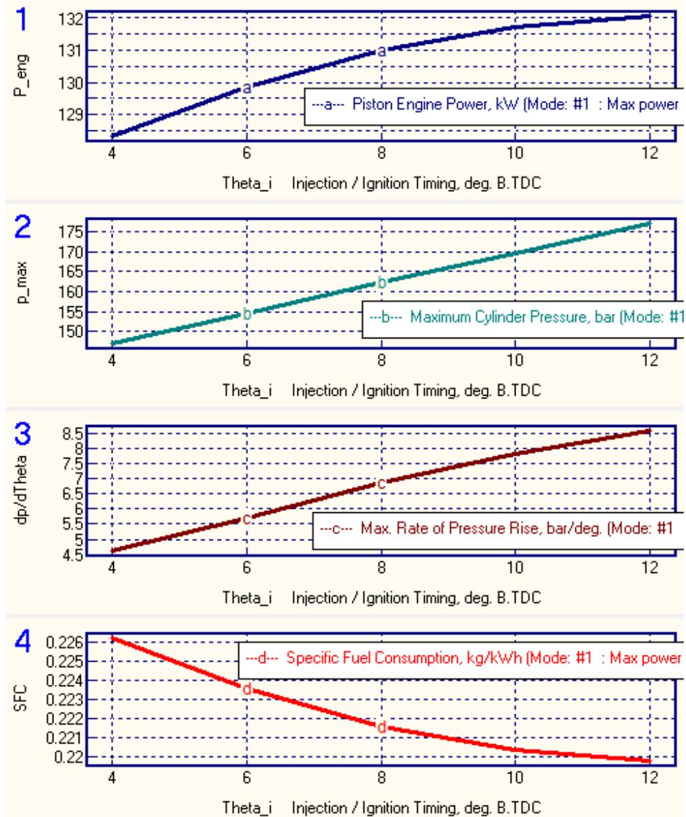
Figure 5. Dependence of the effective power  $P_{eng}$ , the maximum cylinder pressure  $p_{max}$  [bar], the rate of pressure rise  $dp/d\theta$ , and the specific fuel consumption SFC [kg/kWh] on the fuel injection  $\theta_{i}$  at full power mode.
