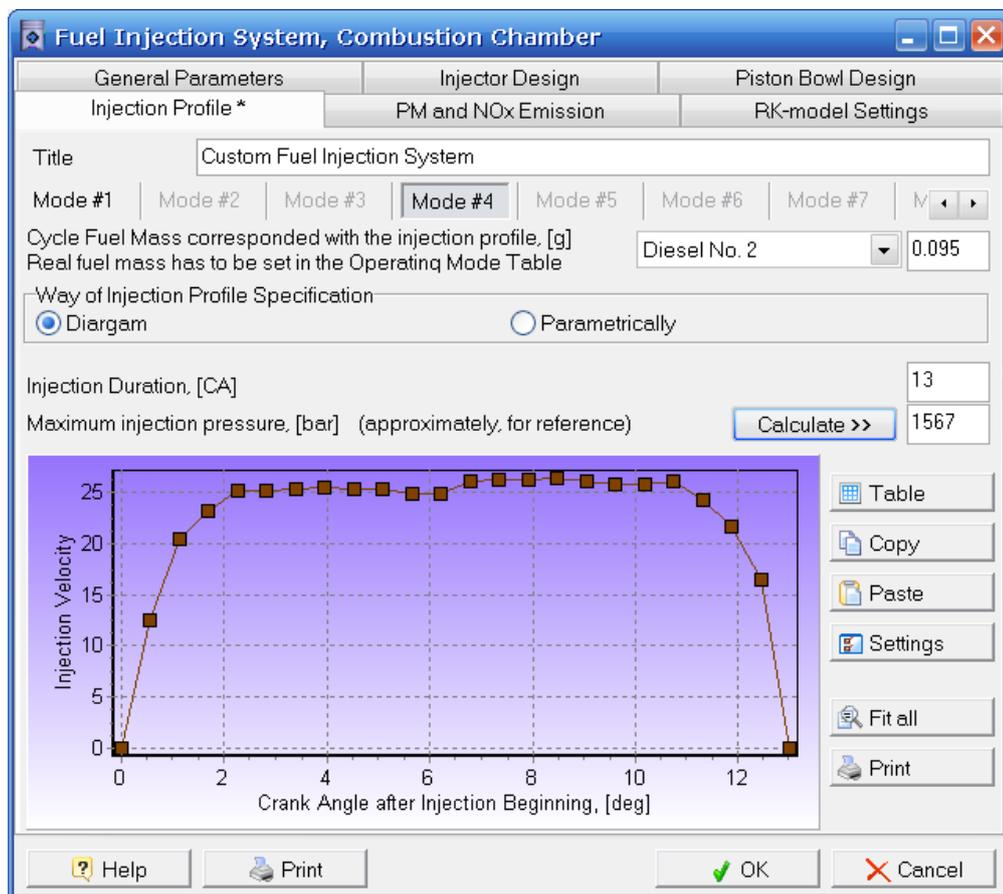
Figure 8. Injection characteristics for intermediate lower power regime (1200 RPM).
